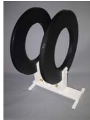
HHS 5204-12 Helmholtz Coil for MIL-STD-461E
